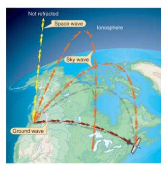
Figure 7-1. Ground, Space, and Sky Wave Propogation.
