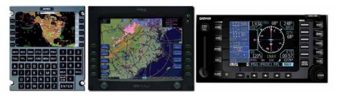
**Figure 7-43.** Typical Display and Control Unit(s) in General Aviation. The Universal UNS-1 (left) controls and integrates all other systems. The Avidyne (center) and Garmin systems (right) illustrate and are typical of completely integrated systems. Although the Universal CDU is not typically found on smaller general aviation aircraft, the difference in capabilities of the CDUs and stand-alone systems is diminishing each year.
