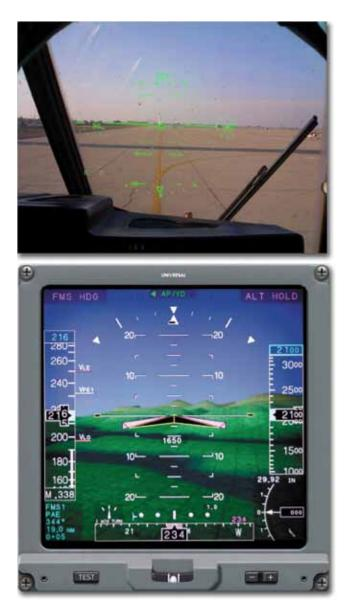
**Figure 7-44.** Example of a Head-Up Display (top) and a Head-Down Display (bottom). The head-up display presents information in front of the pilot along his/her normal field of view while a head-down display may present information beyond the normal head-up field of view.
