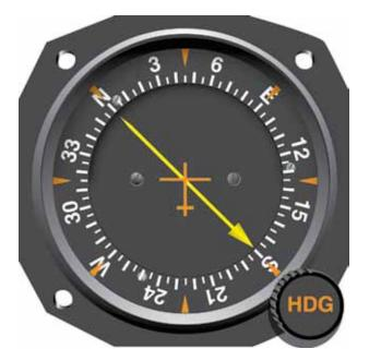
**Figure 7-4.** Relative bearing (*RB*) on a movable-card indicator. By placing the aircraft's magnetic heading (*MH*) of  $045^{\circ}$  under the top index, the relative bearing (*RB*) of  $135^{\circ}$  to the right will also be the magnetic bearing (no wind conditions) which will take you to the transmitting station.
