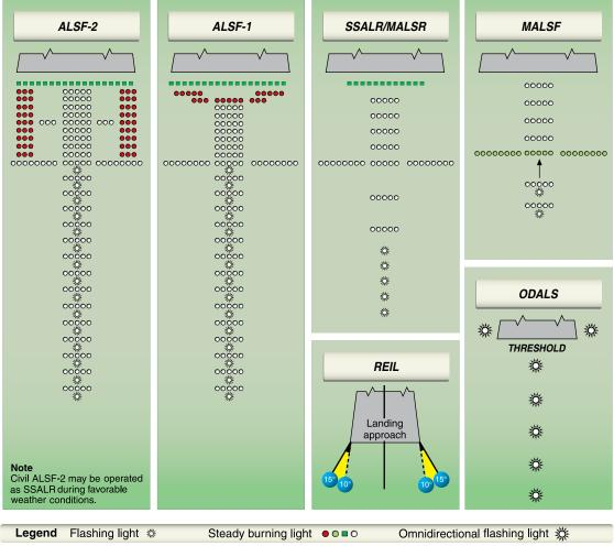
ALSF—Approach light system with sequenced flashing lights
