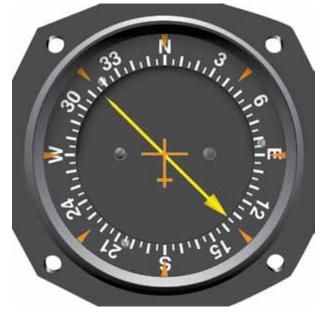
**Figure 7-3.** Relative bearing (*RB*) on a fixed-card indicator. Note that the card always indicates  $360^{\circ}$ , or north. In this case, the relative bearing to the station is  $135^{\circ}$  to the right. If the aircraft were on a magnetic heading of  $360^{\circ}$ , then the magnetic bearing (*MB*) would also be  $135^{\circ}$ .
