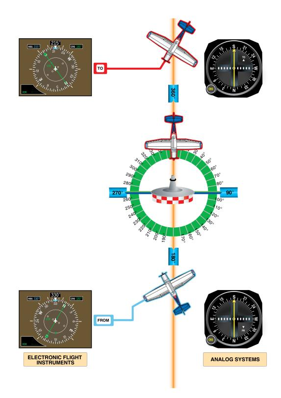
**Figure 7-15.** *CDI Interpretation. The CDI as typically found on analog systems (right) and as found on electronic flight instruments (left).*
