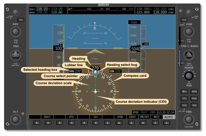
Figure 7-14. An HSI display as seen on the pilot's primary flight display (PFD) on an electronic flight instrument. Note that only attributes related to the HSI are labeled.
