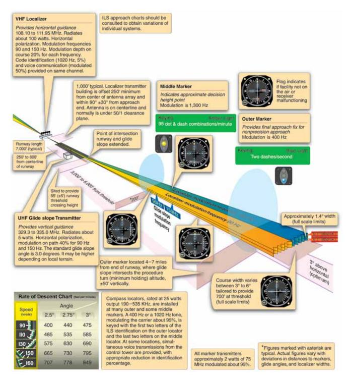
Figure 7-34. Instrument Landing Systems.
