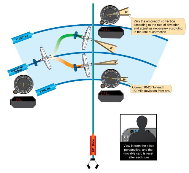
Figure 7-18. Using DME and RMI To Maintain an Arc.
