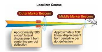
**Figure 7-36.** Localizer receiver indications and aircraft displacement.
